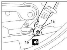
1. Position the end of the front seat belt (1a) on the front seat and tighten the bolt (1b) to the recommended torque.
