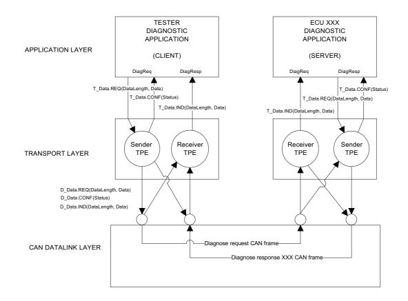
The Diagnostic Application in the Tester prepares a DiagReq message and requests the Sender TPE to transfer the message using the T Data.REQ service primitive.
