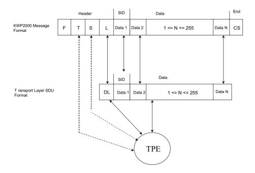
The Format Byte (F) and the Checksum Byte (CS) in the KWP2000 message shall not be transferred at all in the new message structure.
