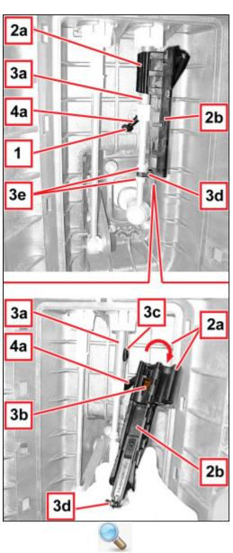
1. Cut the electrical wiring retaining band.
