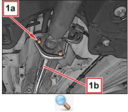
1. Undo the nuts (1a) and disconnect the exhaust pipe (1b) from the flange, then secure it to prevent damage.
