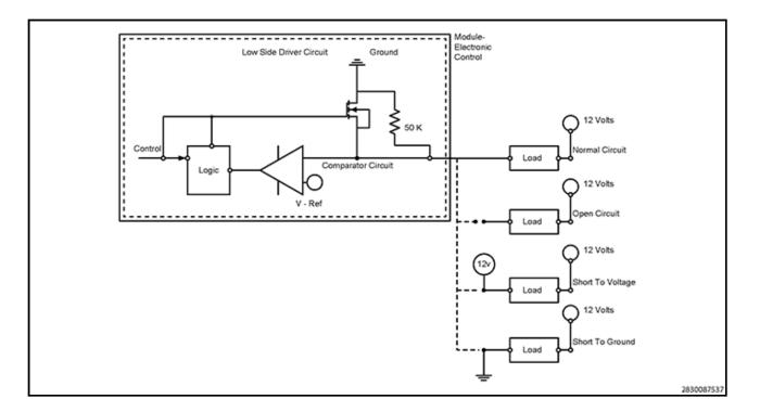
• Circuit Open and Circuit Low Detection: The PCM monitors for an open circuit and short to ground when the driver is switched off. When switched off, the available voltage passes through the device and the internal pull
