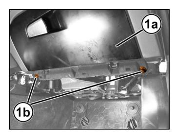
7. Using a trim stick or equivalent, release the retaining clips (1b) and loosen the glove box (3).
