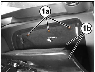
6. Close the glove box door (1a) and remove the screws (1b).
