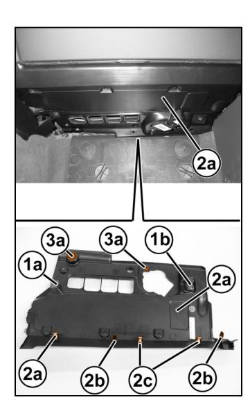
7. Install the instrument panel side cover (1b).
