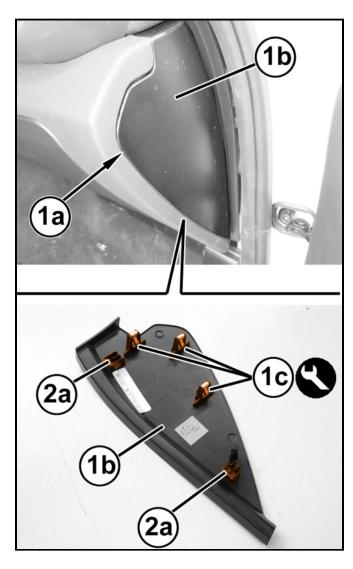
8. Install the floor console front side cover (1a).
