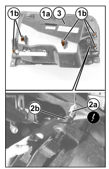
4. Install the screws (1b) and tighten securely.
