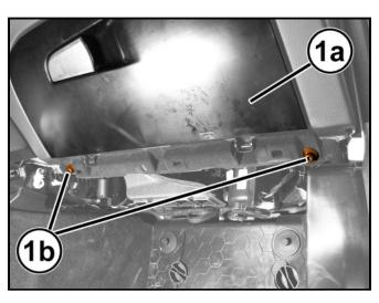
5. Open the glove box door (1b) and install the screws (1a). Tighten the screws securely.
