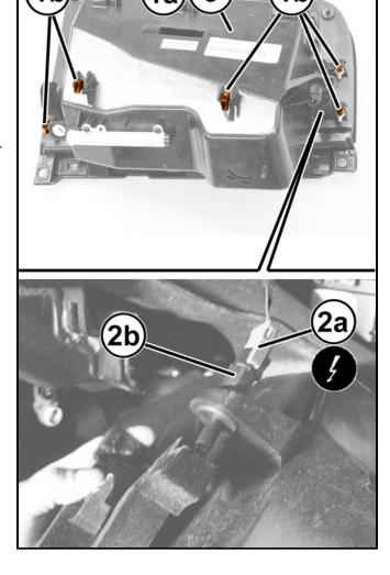
9. If it is necessary to remove the glove box limiter (1c), remove the screws (2a) then remove the rope (1b) from the retainer (1a).
