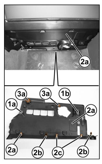
5. Open the glove box door (1b) and remove the screws (1a).
