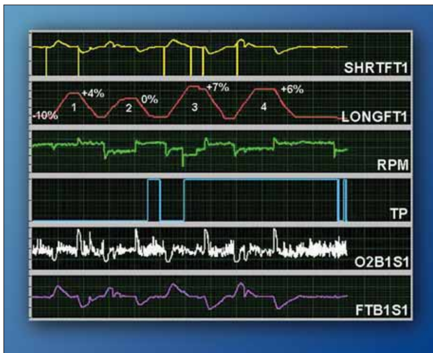
Fig. 5: This is a screen capture from a 2000 Saturn using the ATS EScan Sharpshooter. If the fuel injector connectors are accessible, you can perform an injector balance test using STFT and/or LTFT. The LONGFT1 graph clearly shows a cylinder-to-cylinder difference in injector performance.
