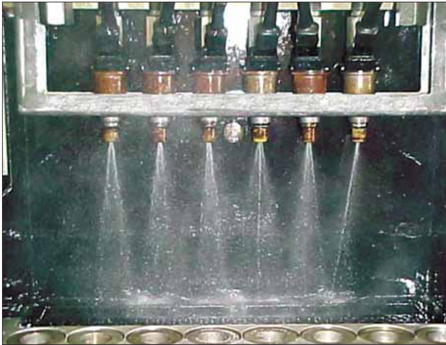
Fig. 2: These fuel injectors from a 2000 Honda Odyssey are being tested by Linder Technical Services on an injector test bench. The injectors have been identified as the likely cause of idle speed and fuel trim issues. Starting from left to right, injectors 4 and 6 exhibit very irregular spray patterns.
