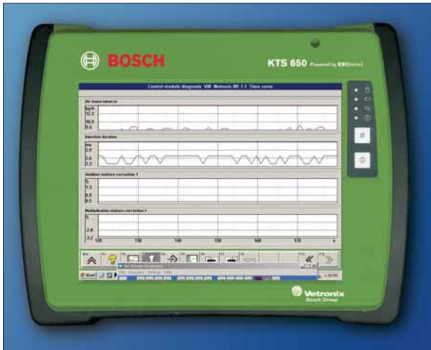
Fig. 7: Volkswagens and Audis have different fuel trim strategies from other manufacturers. Additive Mixture Correction is equivalent to STFT in OBD II generic and changes only at idle speed. Multiplicative Mixture Correction is LTFT in OBD II generic and changes only at cruising speeds. Injection duration changes first for a period of time, then additive and multiplicative will change. It may take as long as 30 seconds before you see any change.
