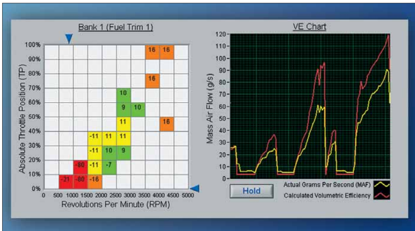
Fig. 6: Diagnosing dirty MAF sensors is a snap with the ATS EScan. This fuel trim map from a 2000 Pontiac GrandAm shows negative fuel trims at idle and positive fuel trims at cruising speed. This is typically how a dirty MAF sensor responds. The MAF overestimates airflow at idle and underestimates it at cruising speeds. The VE chart on the right confirms the diagnosis.
