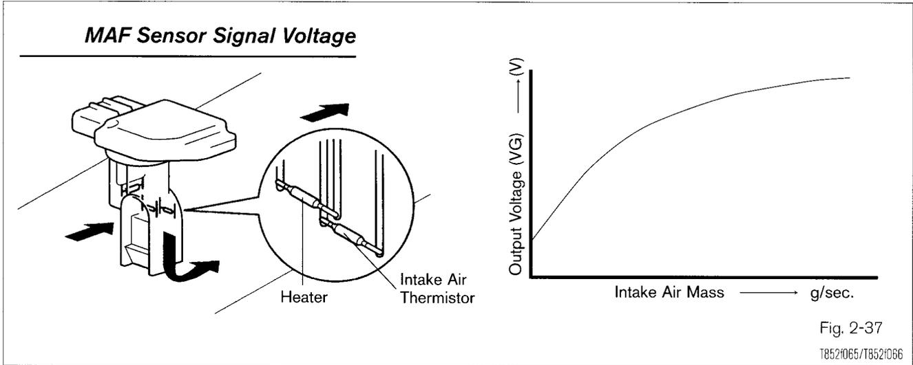
This type of MAF sensor also has an Intake Air Temperature (IAT) sensor as part of the housing assembly. Its operation is described in the IAT section of Temperature Sensors. When looking at the EWD, there is a ground for the MAF sensor and a ground (E2) for the IAT sensor.
