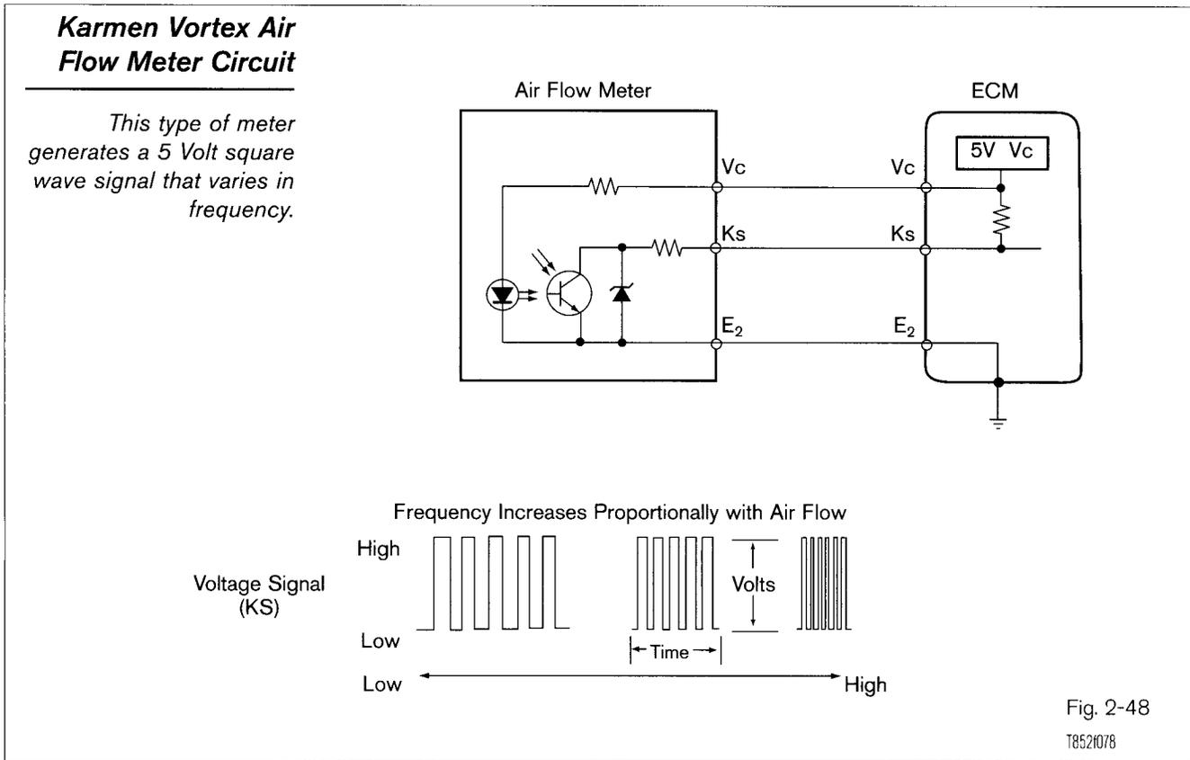
This creates a 5 volt square wave signal that increases frequency in proportion to the increase in intake air flow. Because of the rapid, high frequency nature of this signal, accurate signal inspection at various engine operating ranges requires using a high quality digital multimeter (with frequency capabilities) or oscilloscope.
