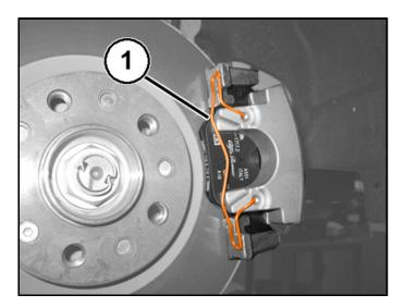
7. Remove the protective cap from the rear brake caliper upper mounting bolt (1).
