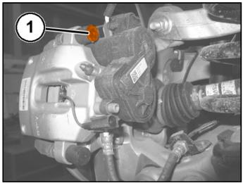
8. Remove the upper caliper to caliper adapter bracket mounting bolt (1).
