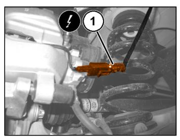
5. Disconnect the electric parking brake (EPB) actuator electrical connection (1) on the rear brake caliper.
