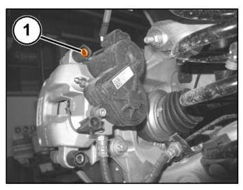
9. Rotate the rear brake caliper on the lower pin.
