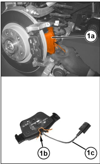
11. Remove the outer brake pad (1).
