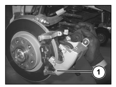
10. Remove the inner brake pad (1a), complete with spring (1b) and electrical harness (1c) of the brake pad wear sensor.
