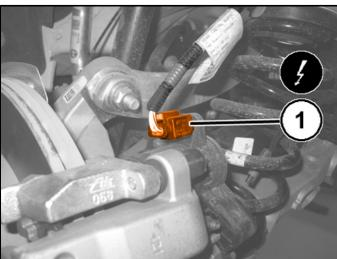
6. Remove the rear brake caliper retaining clip (1).
